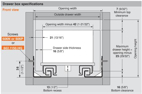
**NOTE**: Drawer side material thickness may vary. Accurate measurement of drawer side material thickness should be used when calculating outside drawer width using the table below. Inside drawer width **must** equal opening width minus **42** (1-21/32") for MOVENTO runners to align and function optimally.
